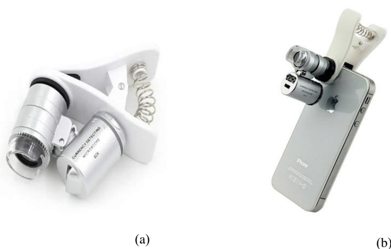
Figure 1 Mobile phone 60 × microscope: (a) a microscope with led lamp and clip, (b) a mobile phone with clipped on 60 × microscope
