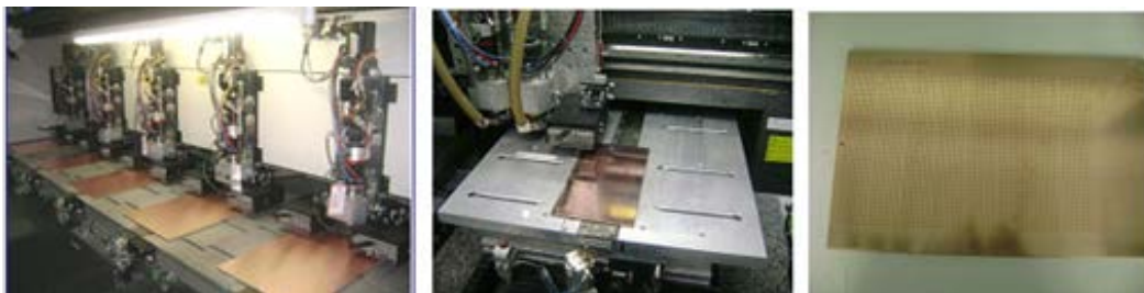
Figure 3 Drilling process and drilled copper plate
