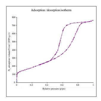
Figure 2 Adsorption-desorption isotherm of the MoS<sub>2</sub> catalyst.
