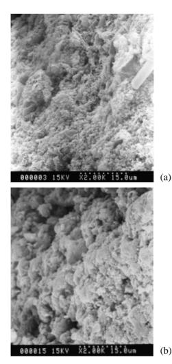
**Figure 4** SEM micrographs of the MoS<sub>2</sub> catalyst (a) before HDS (b) after HDS
