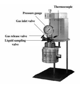
Figure 1 High pressure batch reactor used for the *in situ* decomposition of ammonium thiomolybdate and for hydrodesulfurization.
