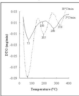
Fig. 3 TPD profiles of phenol on MgO (calcined from Mg(OH)2 at 600°C) by the TG method with a ramp rate of 5°C/min and 30°C/min.
