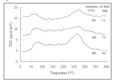
Fig. 2 TPD profiles of phenol on MgO samples using TCD detector.
