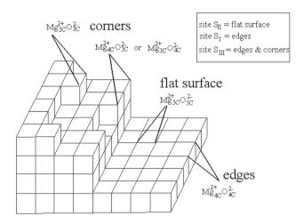
Fig. 8 Model for the low coordination sites on MgO surface.
