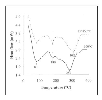
Fig. 4 TPD profiles of phenol desorbed from MgO calcined at 600 and 850°C.
