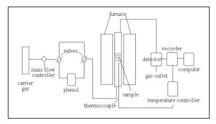
**Fig. 1** TPD apparatus with thermal conductivity detector(TCD).
