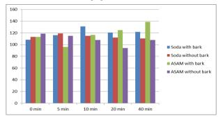
Figure 2. Histogram of grammage (g/m<sup>2</sup>) vs beating time, min for soda and ASAM pulps.
