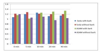
Figure 1. Histogram average weight (grams) vs beating time, min for soda and ASAM pulps.
