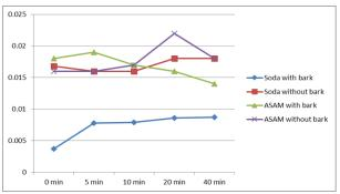
Figure 5. Burst index (k Pa m<sup>2</sup>/g) vs beating time (min) for soda and ASAM pulps.
