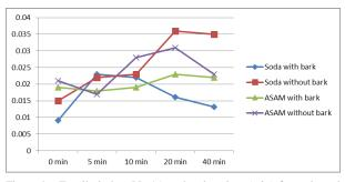
Figure 4. Tensile index (Nm/g) vs beating time (min) for soda and ASAM pulps.
