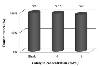
Figure 5. Effect of NH<sub>4</sub>OH catalyst concentration on transmittance at 625 nm by UV/VIS Spectrophotometer.
