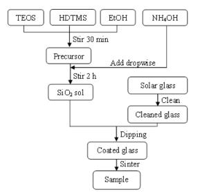
Figure 1. Procedure for making coated glass samples
