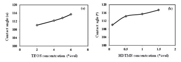
Figure 3. The water-contact angles tested by varying the concentration of )a( TEOS, and )b( HDTMS, on preparing the coating.
