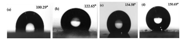
Figure 4. Photographs of water droplets with associated contact angles on the coated glass surfaces. )a( Treated with 0.05% NH<sub>4</sub>OH, )b( treated with 0.1% NH<sub>4</sub>OH, )c( treated with 0.5% NH<sub>4</sub>OH, and )d( treated with 1.0% NH<sub>4</sub>OH.
