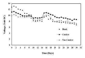
Figure 7. Time traces of solar cell voltage during outdoor exposure for up to 30 days of coated and uncoated solar cells.
