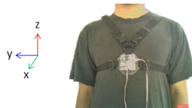
Figure 1. Position of the tri-axial accelerometer.
