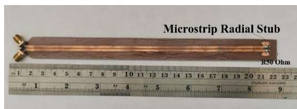
Fig. 8 The sensor model of the parallel-coupled microstrip lines for water level measurement.
