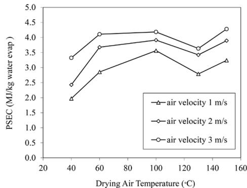
**Figure 8. Primary specific energy consumption (PSEC) when using resting period of 1 min**
