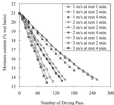
Figure 5. Reduction of paddy moisture content at drying air temperature 150°C
