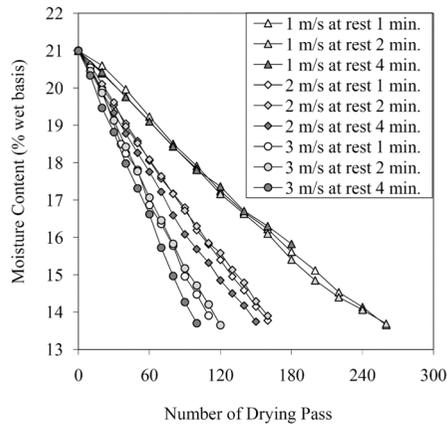
Figure 4. Reduction of paddy moisture content at drying air temperature 130°C
