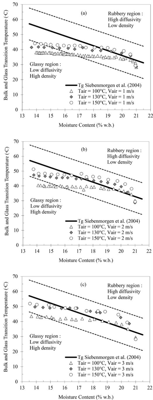
Figure 7. Bulk paddy temperature at rest period of 1 min on state diagram
