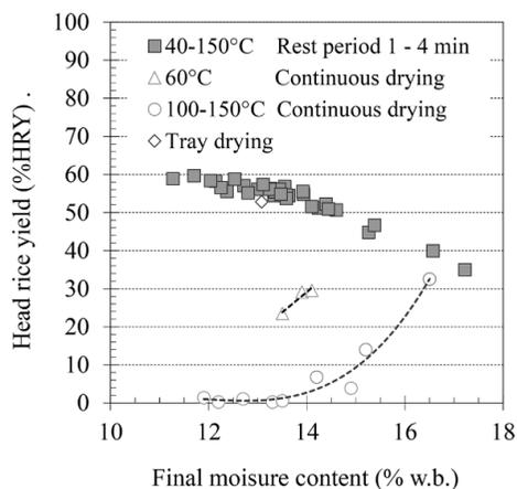
**Figure 9. Relationship between head rice yield and final moisture content before milling**
