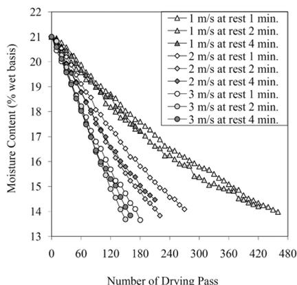
Figure 3. Reduction of paddy moisture content at drying air temperature 100°C
