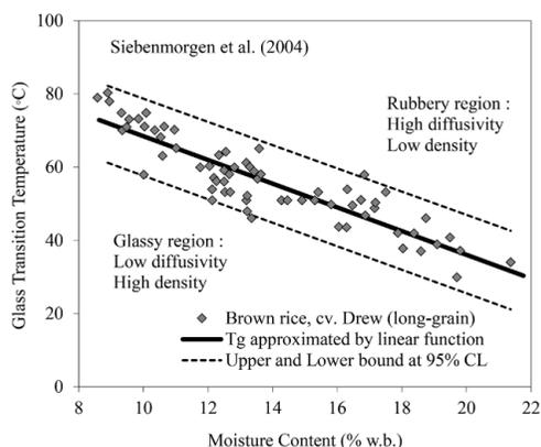
**Figure 2. Glass transition temperatures vs. moisture contents for brown rice kernels (cv. Drew) (Seibenmorgen *et al.*, 2004)**
