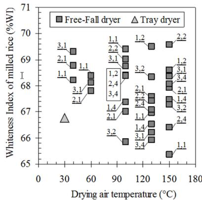
**Figure 11. Whiteness index of milled rice under any drying condition**
