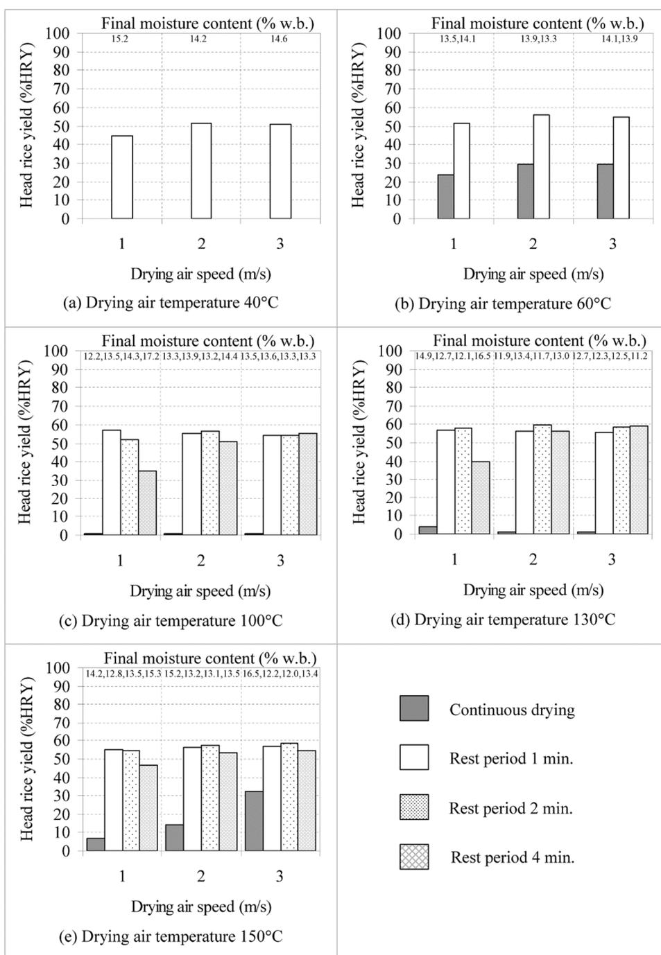
Figure 10. Head rice yield and final moisture content under any drying condition
