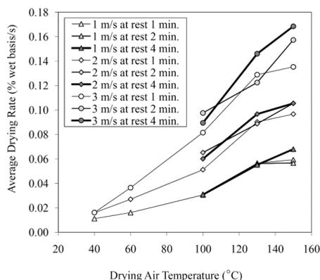
**Figure 6.** The effect of temperatures, air velocities, and rest periods to the average drying rate
