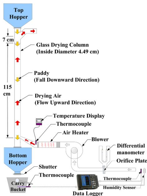
**Figure 1. Schematic of the laboratory-scale free-fall dryer**
