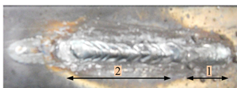
Figure 6. The weld result when arc-voltage controlled within 1.5 V – 2.8 V
