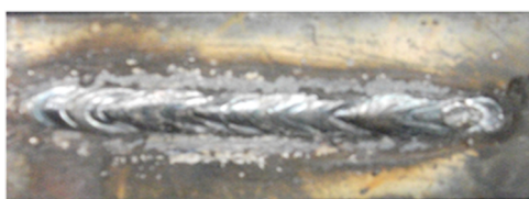
Figure 8. The weld result when arc-voltage controlled within 1.5 V – 2.5 V
