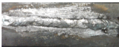
Figure 12. The weld result when arc-voltage controlled within 1.5 V – 1.9 V
