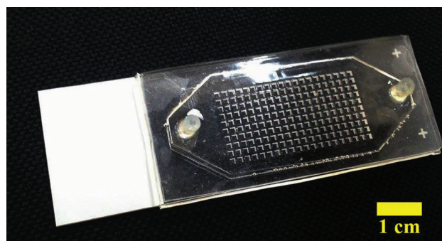
Figure 3. The image of the fabricated biochip is shown. The device is microscope slide size and clear for cell observation through a microscope. The scale bar represents a length of \sim 1 cm
