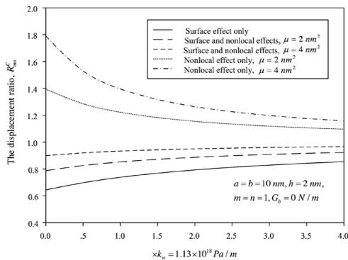
Figure 6. Variation of the displacement ratio as the Winkler foundation stiffness for the classical plate
