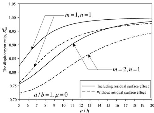
Figure 4. The effect of residual surface tension on the displacement ratio for the classical plate with different half-wave numbers
