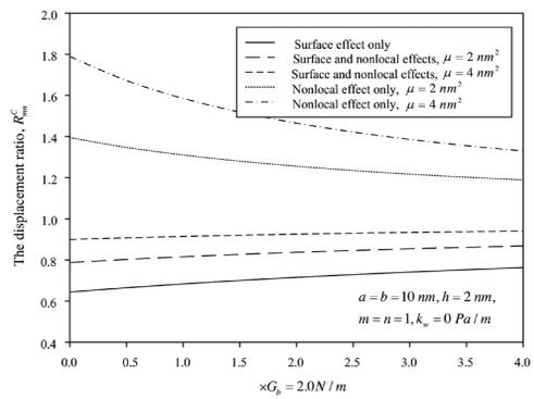
Figure 7. Variation of the displacement ratio as the shear layer stiffness for the classical plate
