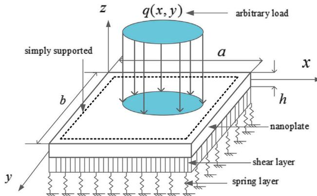
Figure 1. Geometric of a uniform rectangular nanoplate embedded in elastic medium
