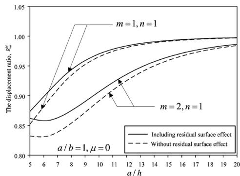
Figure 5. The effect of residual surface tension on the displacement ratio for the Mindlin plate with different half-wave numbers
