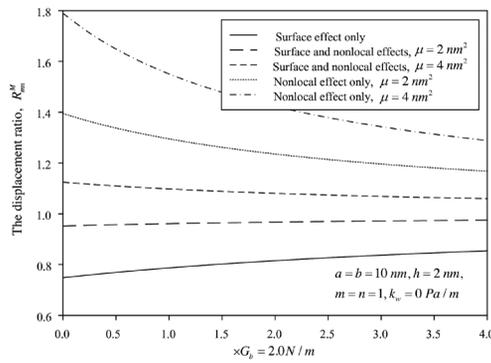
Figure 9. Variation of the displacement ratio as the shear layer stiffness for the Mindlin plate
