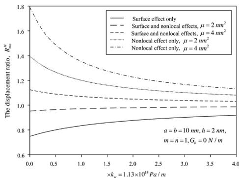
Figure 8. Variation of the displacement ratio as the Winkler foundation stiffness for the Mindlin plate
