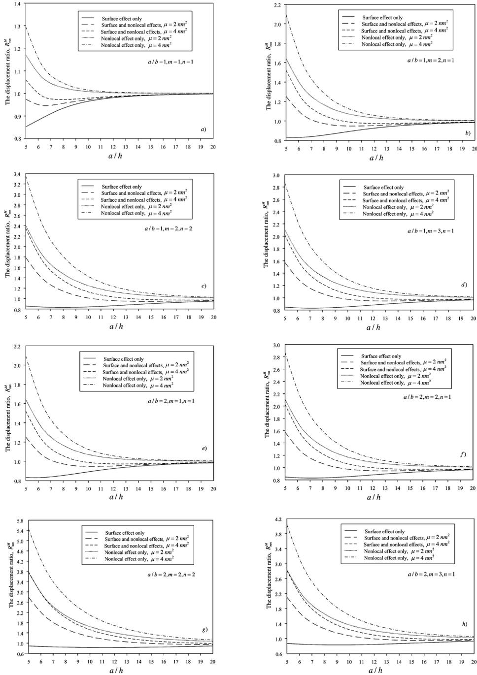
Figure 3(a)-(h). Variation of the displacement ratio as a non-dimensional length of nanoplates for the Mindlin plate with different length-to-width ratio and half-wave numbers
