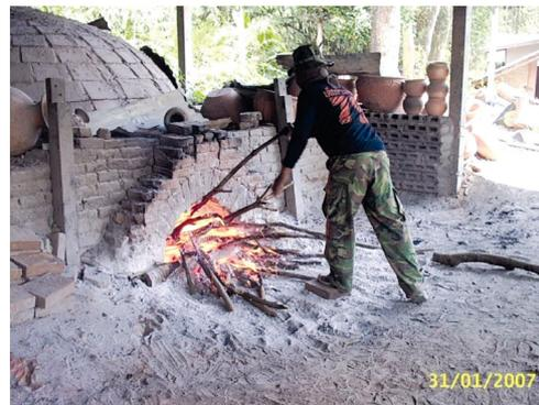
Figure 2. A kiln operator loading wood into a Dan Kwian kiln
