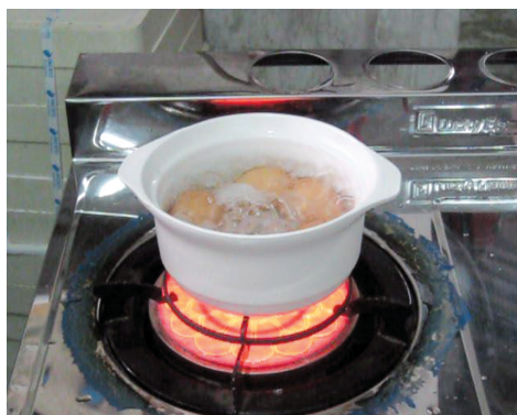
Figure 4. The cooking test of the cordierite pot glazed with L2.9
