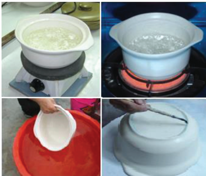
Figure 3. The test on a hot plate and a gas stove-top of the cordierite pot glazed with L2.9
