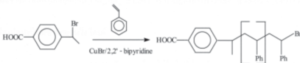
Figure 2. Synthesis of carboxylic acid terminated polystyrene by ATRP (Malz et al. , 1999).
