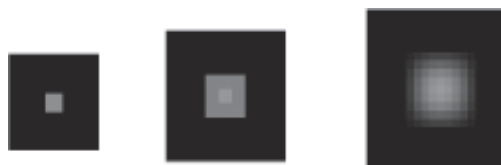
Figure 3. Target matrix for test resolution at 60, 30 and 15 \mu\text{m} .
