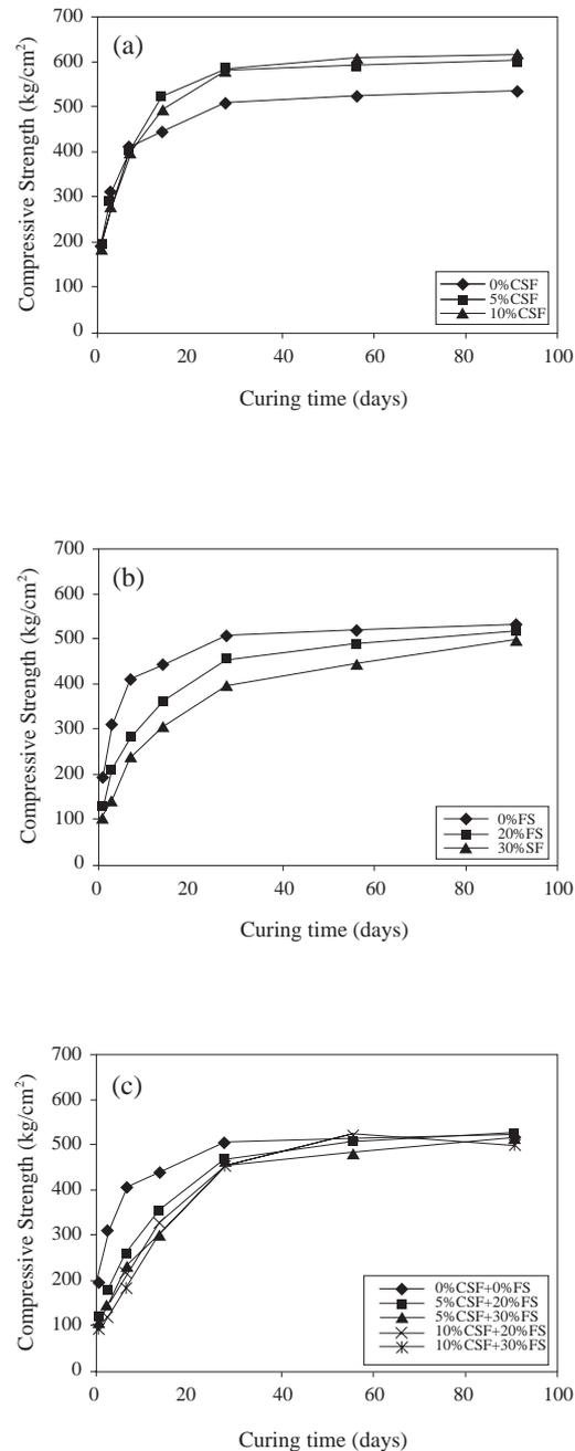
**Figure 1. Compressive strength of the blended cement pastes at increasing curing time: (a) OPC + CSF; (b) OPC + FS; and (c) OPC + CSF + FS**
