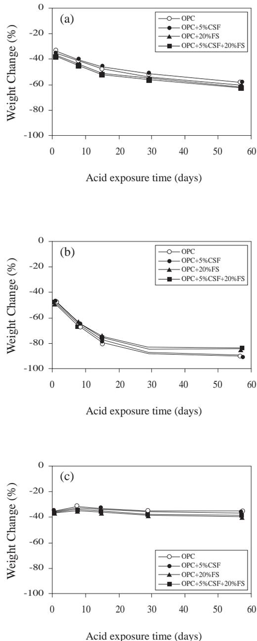
**Figure 3.** Weight change of the solidified waste sample containing 20% (w/w) plating sludge after exposure to acid solutions: (a) acetic; (b) nitric; and (c) sulfuric
