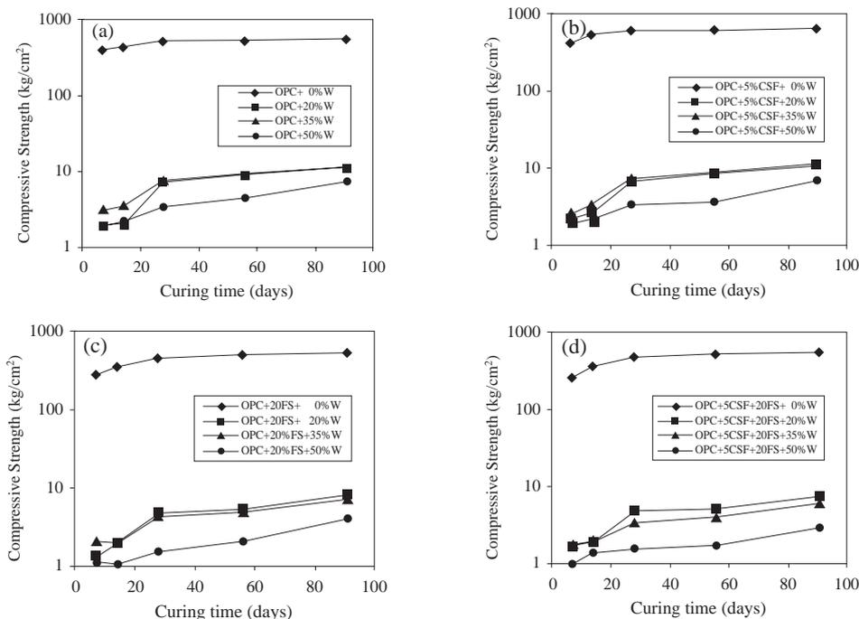
**Figure 2. Compressive strength of the solidified wastes containing various waste loading concentrations; (a) OPC; (b) OPC + 5%CSF, (c) OPC = 20%FS; and (d) OPC + 5%CSF + 20%FS**
