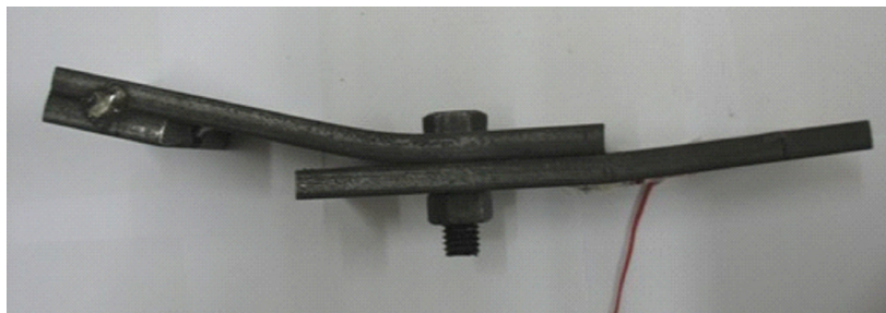
Figure 15. Deformation of specimen after 15 kN bending force
