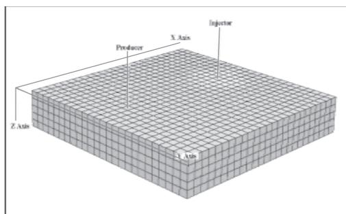
Figure 4. Geometry of reservoir model and well locations
