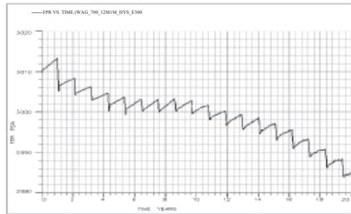
Figure 7. Pressure of reservoir vs. Time plot of 700 RB/D
