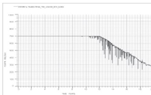
Figure 5. Oil production rate vs. Time plot of 700 RB/D
