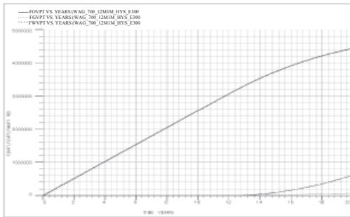
Figure 6. Cumulative fluid production vs. Time plot of 700 RB/D
