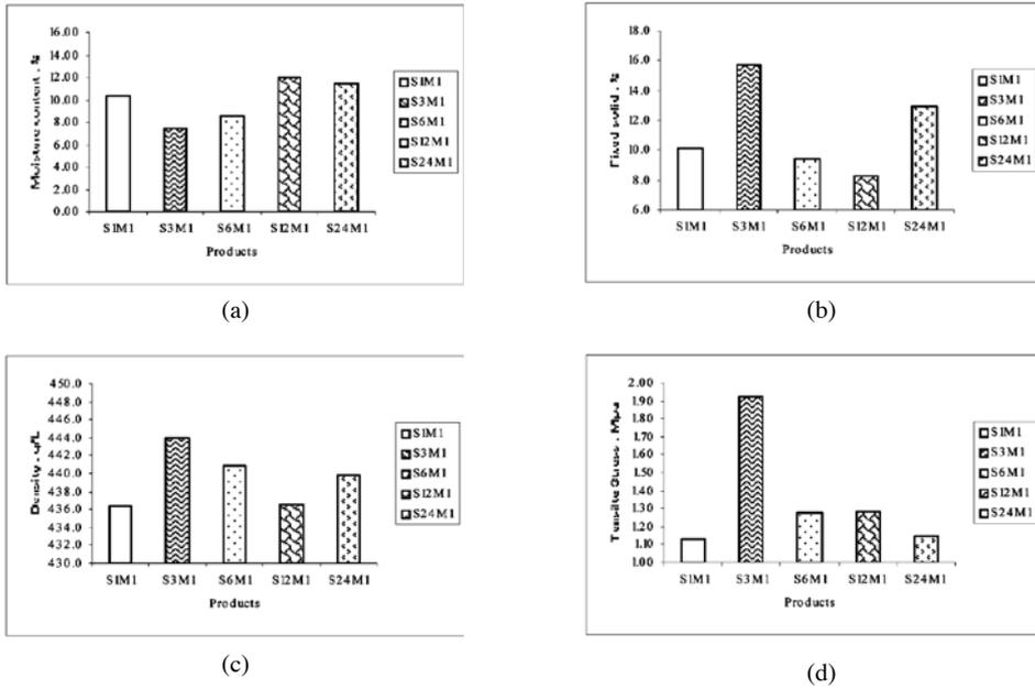
Figure 11. Characterisation of paperboard briquette products at a constant molding period 1 h and varied soaking time (1, 3, 6, 12, and 24 h).
