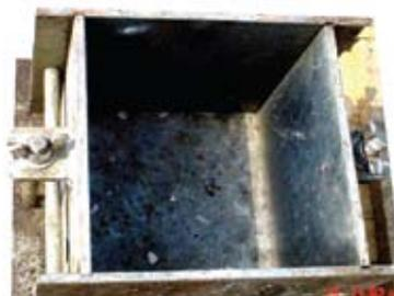
**Figure 5. A specimen setting mold in this study for production of paper-board briquette products**
