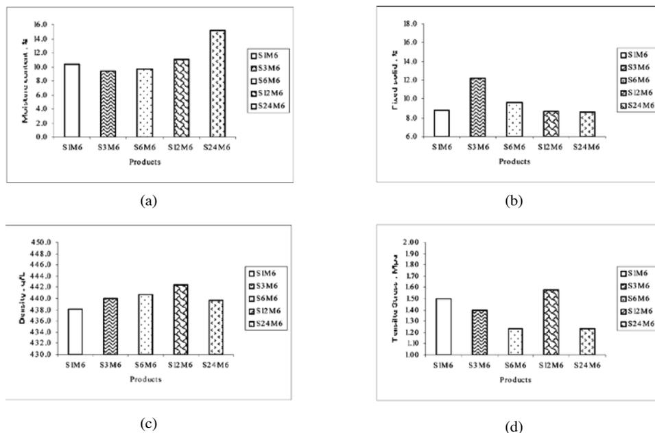
**Figure 13. Characterisation of paperboard briquette products at a constant molding period 6 h and varied soaking time (1, 3, 6, 12, and 24 h). (a) Moisture Content (b) Fixed Carbon (c) Bulk Density (d) Tensile Stress**
