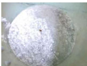
**Figure 4. An example of homogenous paper pulp sample to be used as raw material for production of paperboard briquette products**
