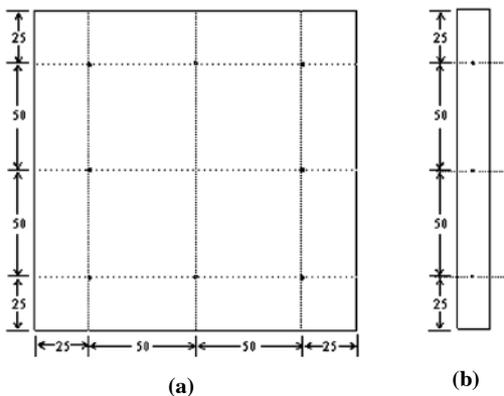
Figure 8. Points at which lengths, widths and thicknesses (mm) of test pieces were measured (a) Planview (b) Side view
