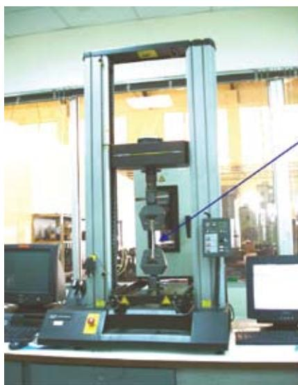
Position of test pieces as installed for testing tensile stress measurements
