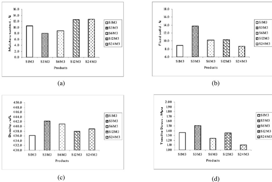
Figure 12. Characterisation of paperboard briquette products at a constant molding period 3 h and varied soaking time (1, 3, 6, 12, and 24 h).
