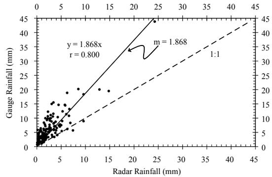
**Fig. 2** Scatter plot of mean radar rainfall and mean gauge rainfall based on the relationship  $Z = 200R^{1.6}$ .
