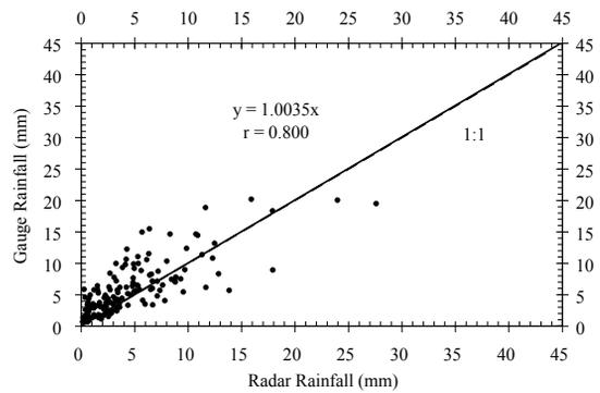
**Fig. 3** Scatter plot of mean radar rainfall and mean gauge rainfall based on the relationship  $Z = 74R^{1.6}$ .
