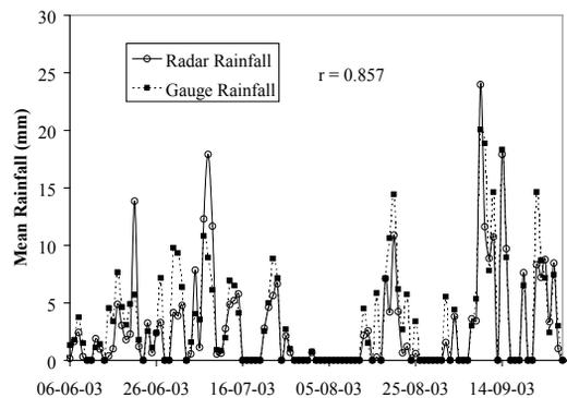
**Fig. 4** Time series plot of mean gauge rainfall and radar rainfall in 2003 using the relationship  $Z = 74R^{1.6}$ .
