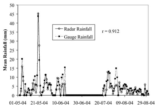
Fig 5. Time series plot of mean gauge rainfall and radar rainfall in 2004 using the relationship  $Z = 74R^{1.6}$ .
