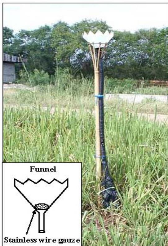
Fig 1. The photograph of an air particulate collector.
