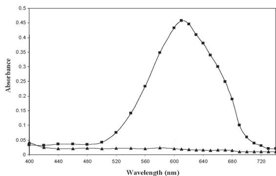
**Fig 1.** Absorption spectra of the reaction product of Fe<sup>3+</sup> + AAP + IDB (—■—) and reagent blank (---▲---).
