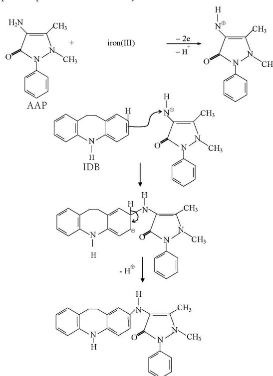
**Fig 2.** Proposed mechanism of the reaction between AAP and IDB.
