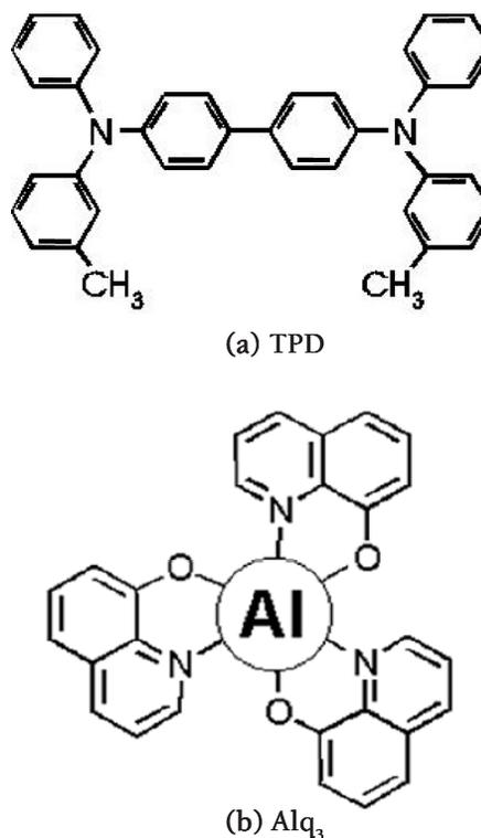
Fig 1. Chemical Structure of (a) TPD, (b) Alq<sub>3</sub>.
