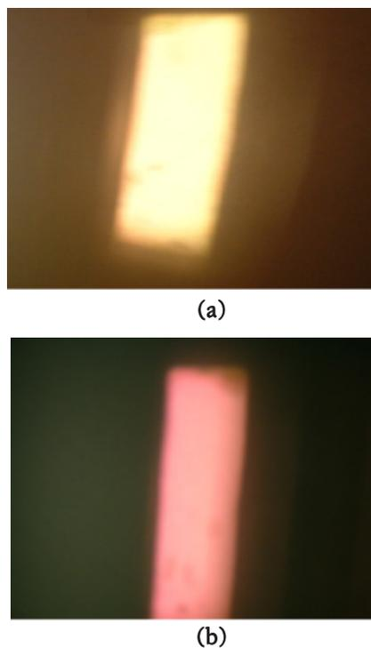
**Fig 3.** Room temperature-Luminescence color from structure A with: (a) 20-nm thick Alq<sub>3</sub> layer; (b) 50-nm thick Alq<sub>3</sub> layer.
