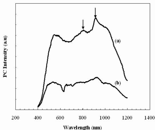
**Fig 6.** Photocurrent of structure B with different TPD thickness (a) 100 nm thick, (b) 5 nm thick.
