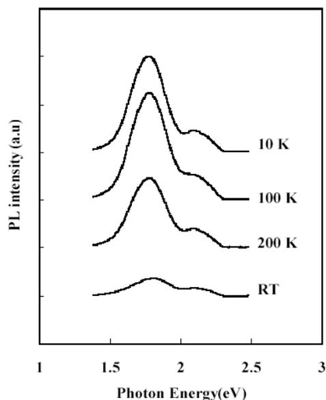
**Fig 5.** Temperature dependent PL of structure A with 10 nm-well width.
