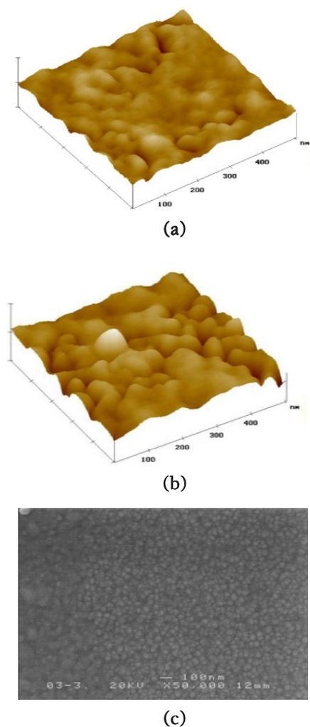
**Fig 2.** (a) AFM images of surface morphology of Alq<sub>3</sub> thin films with thickness of 15 nm; (b) with thickness of 50 nm; (c) SEM image of ZnSe layer.
