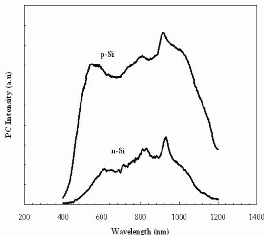
**Fig 7.** Photocurrent of structure B on different type of Si substrate.
