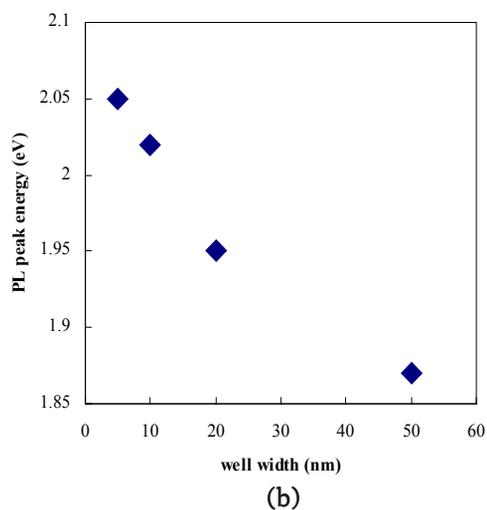
**Fig 4.** (a) Room temperature-PL of structure A with different well thickness as function of photon energy. (b) Room temperature-PL peak photon energy of structure A as a function of well thickness.
