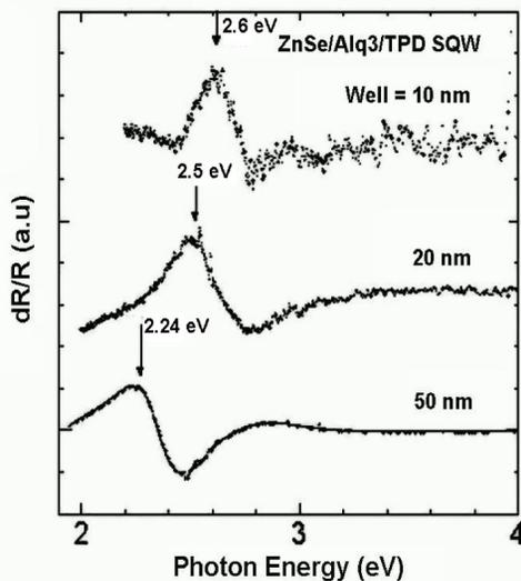
**Fig 8.** Room temperature-ER spectra of structure B as a function of the well thickness. The arrows indicate the transition energies determined by the fittings.
