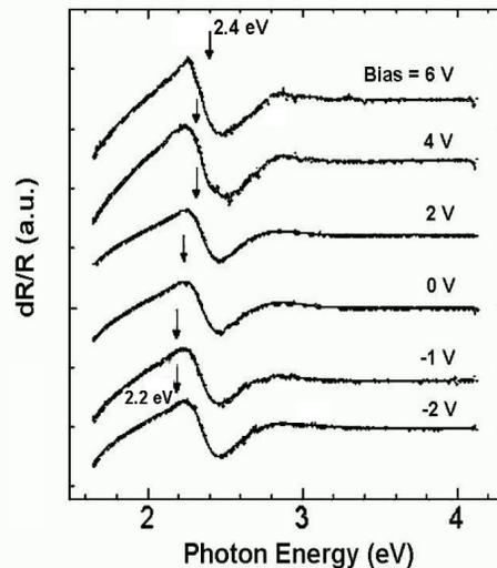
**Fig 9.** ER spectra of structure B with 50-nm Alq<sub>3</sub> layer measured in applied voltage +6.0 ~ -2.0V.
