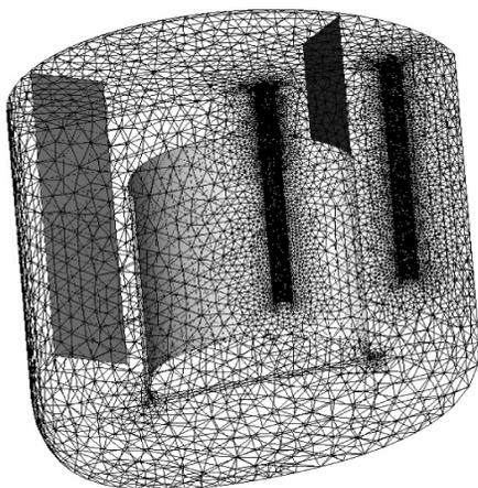
Fig 3. Generated volume mesh for the crystallizer model.
