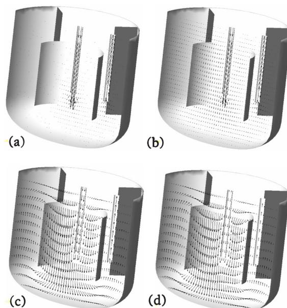
Fig 4. Velocity vectors for one half of the tank for momentum source additions of (a) 0 kg/m<sup>2</sup>/s<sup>2</sup>; (b) 1000 kg/m<sup>2</sup>/s<sup>2</sup>; (c) 18000 kg/m<sup>2</sup>/s<sup>2</sup>; (d) 50000 kg/m<sup>2</sup>/s<sup>2</sup>.
