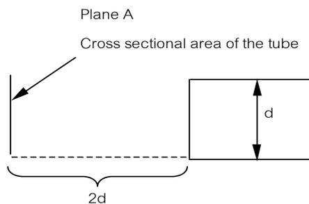
**Fig 8.** Location of the plane used to check for the isokinetic flow condition.
