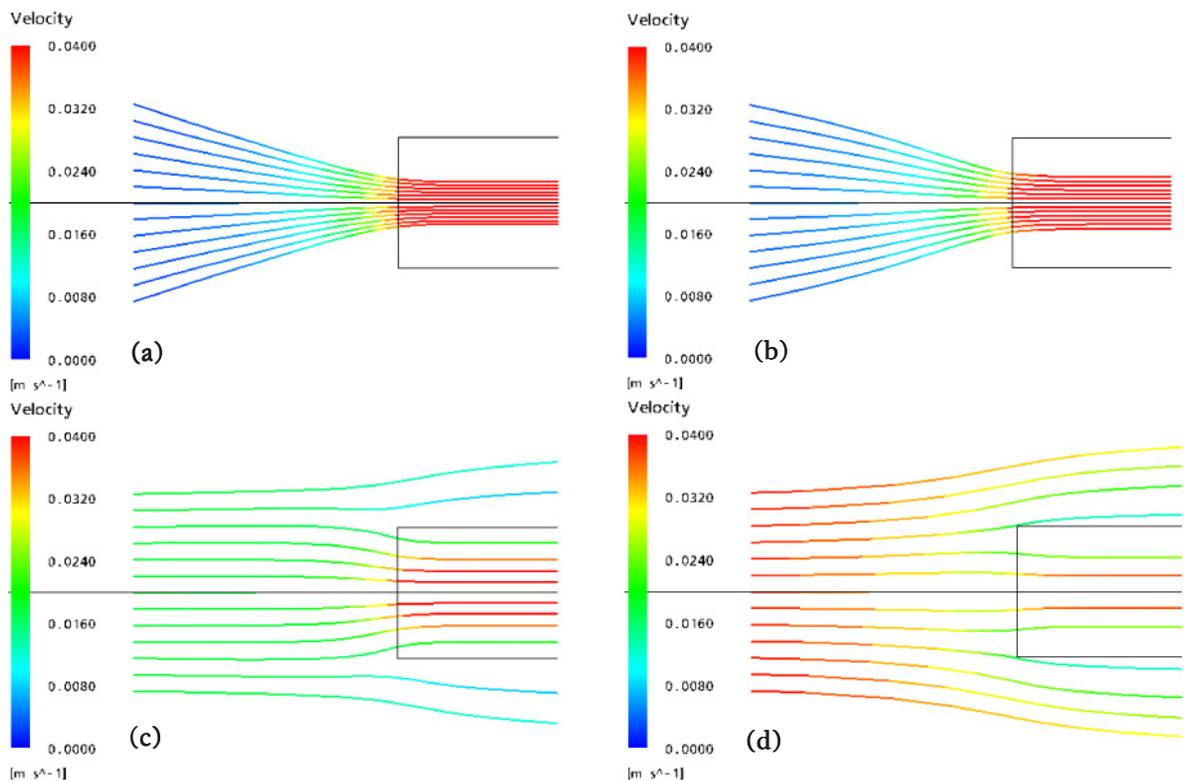
**Fig 6.** Streamlines around the outlet tube for momentum source additions of (a) 0 kg/m<sup>2</sup>/s<sup>2</sup>; (b) 1000 kg/m<sup>2</sup>/s<sup>2</sup>; (c) 18000 kg/m<sup>2</sup>/s<sup>2</sup>; (d) 50000 kg/m<sup>2</sup>/s<sup>2</sup>.
