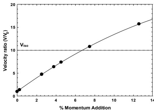
**Fig 9.** Velocity at a plane near the outlet of the crystallizer as a function of the amount of momentum added by the impeller.
