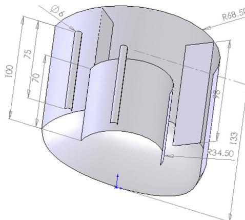
Fig 1. Schematic model of the experimental crystallizer.
