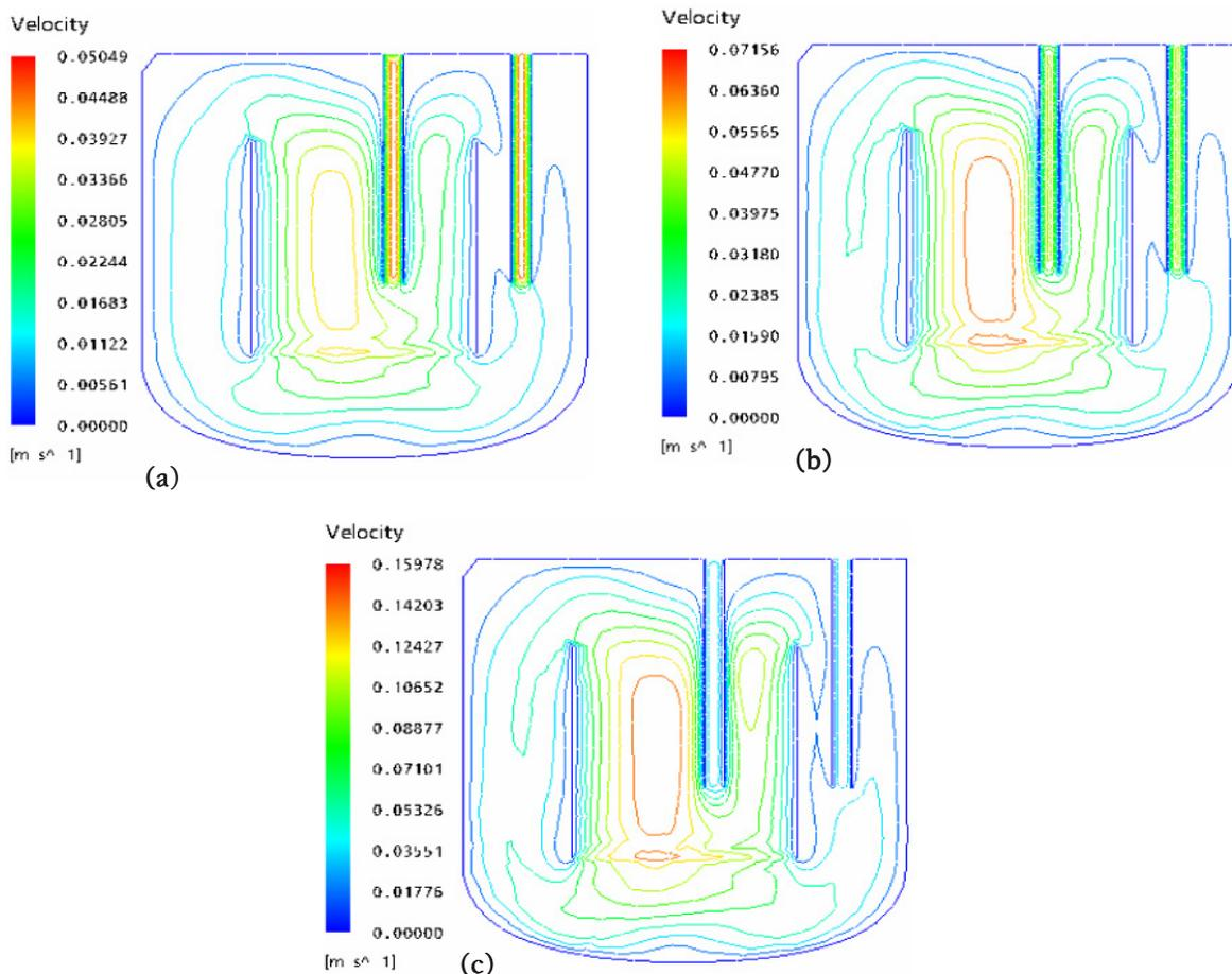
**Fig 7.** Velocity contour plots at the tank centerline for momentum source additions of (a) 10000 kg/m<sup>2</sup>/s<sup>2</sup>; (b) 18000 kg/m<sup>2</sup>/s<sup>2</sup>; (c) 50000 kg/m<sup>2</sup>/s<sup>2</sup>.
