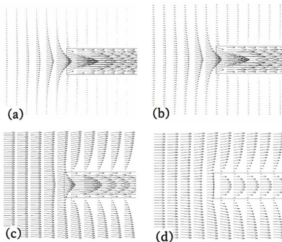
**Fig 5.** Velocity vectors around the outlet tube for momentum source additions of (a) 0 kg/m<sup>2</sup>/s<sup>2</sup>; (b) 1000 kg/m<sup>2</sup>/s<sup>2</sup>; (c) 18000 kg/m<sup>2</sup>/s<sup>2</sup>; (d) 50000 kg/m<sup>2</sup>/s<sup>2</sup>.
