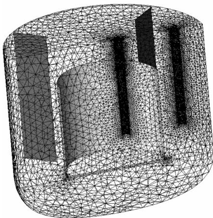
**Fig 3.** Generated volume mesh for the crystallizer model.
