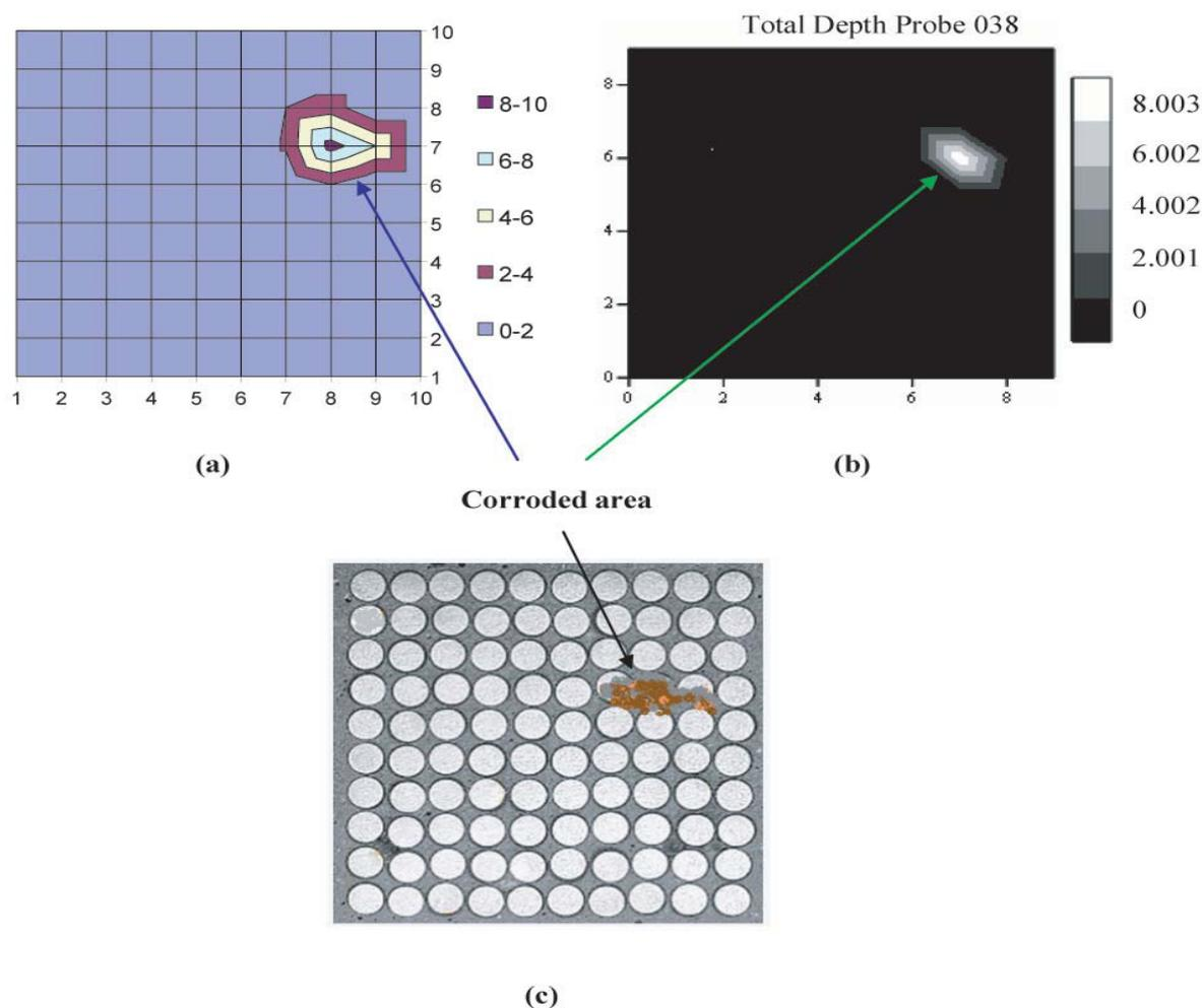
**Fig 5.** (a) Observed pitting corrosion depth map, (b) Calculated pitting corrosion depth map values (in mm) and (c) the photograph showing a carbon steel WBE surface after exposure to Evans solution for 17 hrs.
