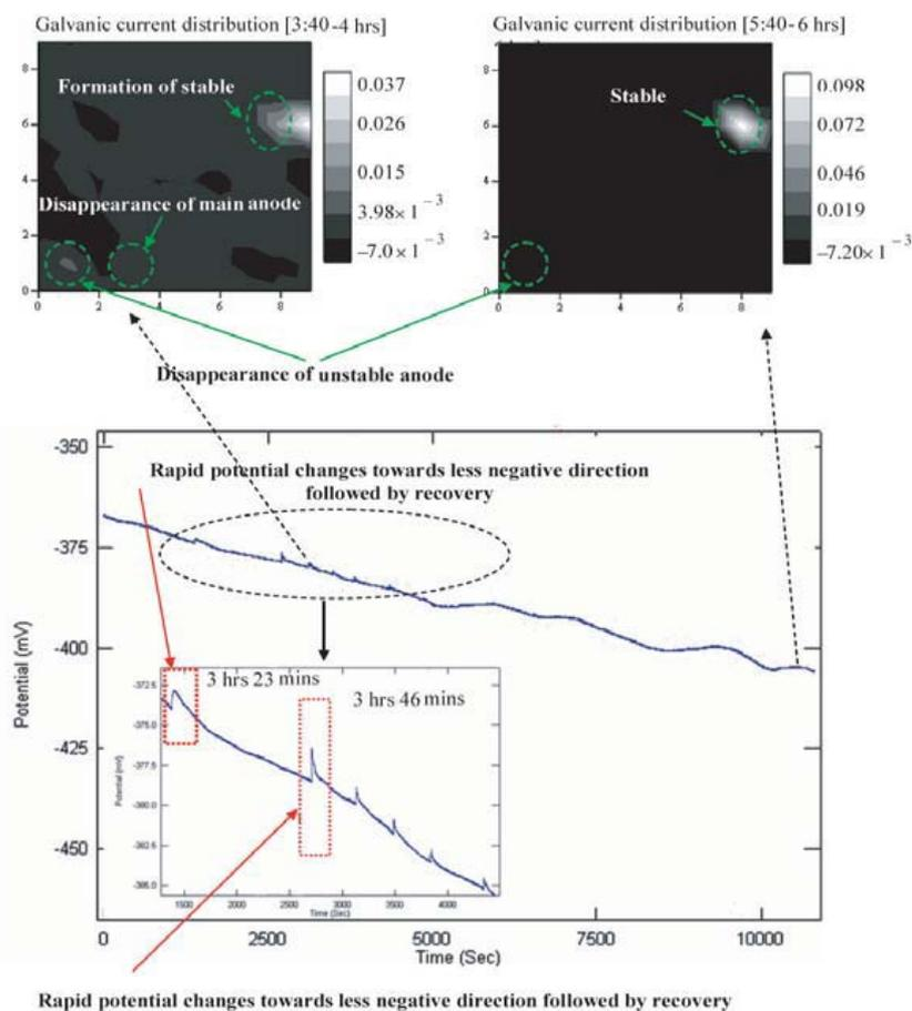
**Fig 3.** Correlation of potential noise signature and galvanic current ( $\text{mA}/\text{cm}^2$ ) distribution map obtained from a carbon steel WBE showing pitting initiation, repassivation and stable pit formation stage after exposure to Evans solution for 6 hours.
