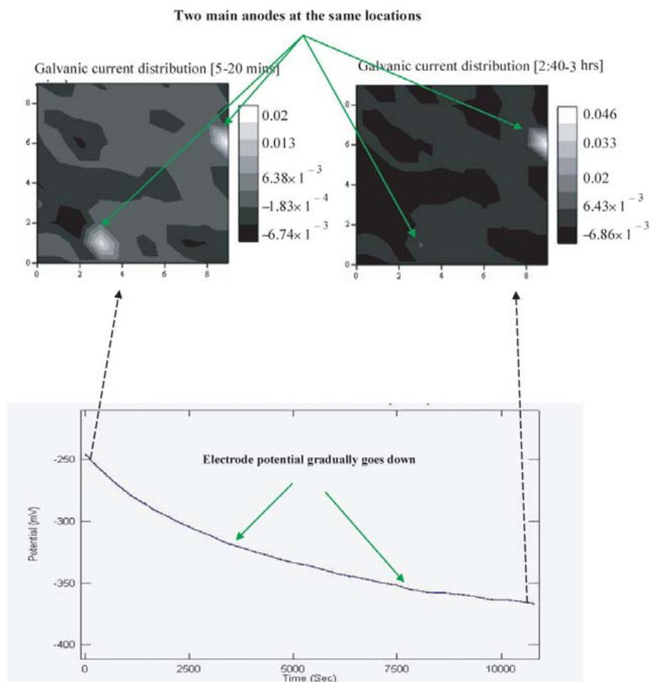
**Fig 2.** Correlation of potential noise signature and galvanic current (mA/cm<sup>2</sup>) distribution map obtained from a carbon steel WBE showing the first stage prior to pitting after exposure to Evans solution for 3 hours.
