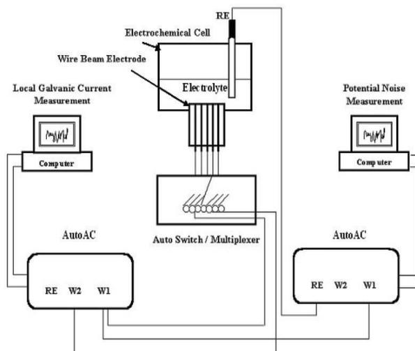
**Fig 1.** Schematic diagram showing an experimental set-up for detecting potential noise over a WBE and for mapping galvanic currents flowing into/out of each wire in the WBE from pitting corrosion system.
