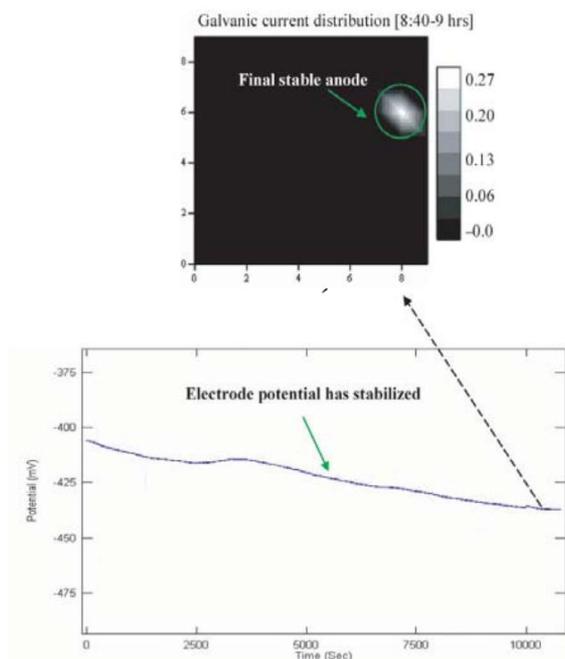
**Fig 4.** Correlation of potential noise signature and galvanic current ( $\text{mA}/\text{cm}^2$ ) distribution map obtained from a carbon steel WBE showing stabilization stage of pitting after exposure to Evans solution for 9 hours.
