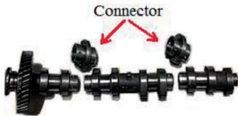
Fig. 3 The modified intake camshaft for 5-stroke engine
