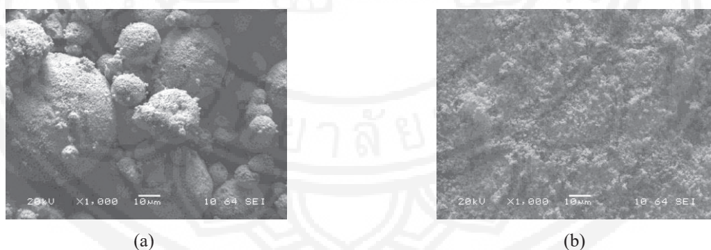
Figure 3 SEM micrographs of PZT 5H powder: (a) as-received and (b) after vibro-milling for 48 hrs
