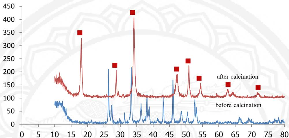
**Figure1** Powder XRD patterns: Golden apple snail shell before calcinations and calcium oxide after calcinations (■ as calcium oxide).
