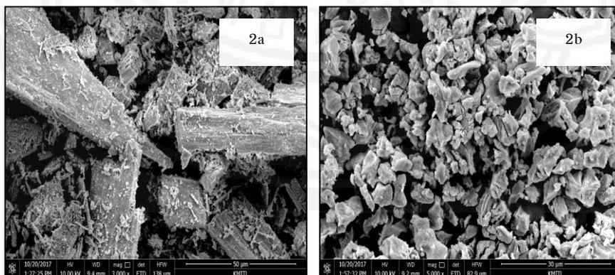
**Figure2** SEM images of (2a) Golden apple snail shell and (2b) Calcium oxide.
