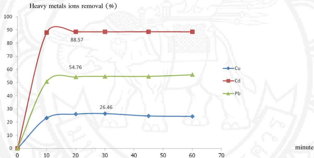
**Figure 3** Effect of contact time on heavy metal ion removal (dose 0.5 g, ion concentration 1 mg/L, pH 6)
