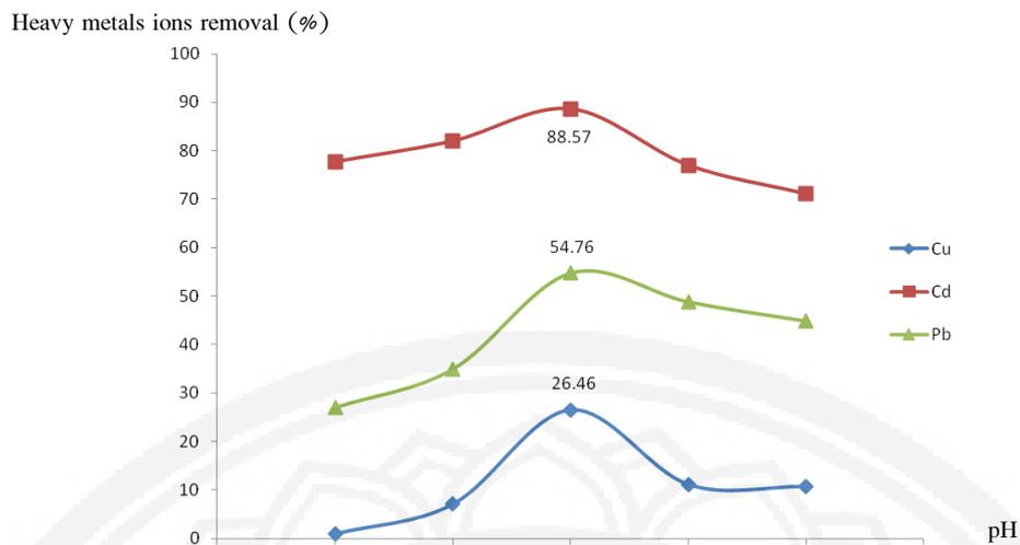
Figure4 Effect of pH on heavy metals ions removal(dose 0.5 g, metal ion concentration 1 mg/L, 30 min)
