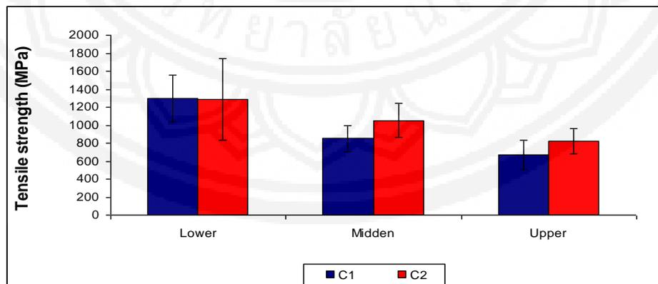
Figure 4 The tensile strength of C1 and C2 culms
