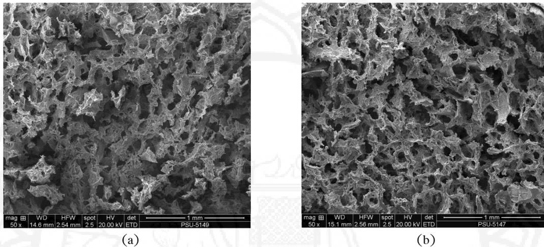
Figure 2 SEM micrographs a) PSC coated chitosan scaffold b) chitosan scaffold
