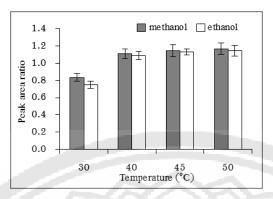
Figure 4 Effect of incubation and extraction temperatures on peak area ratio of methanol and ethanol. Error bar was 1S.D. (n = 3).
