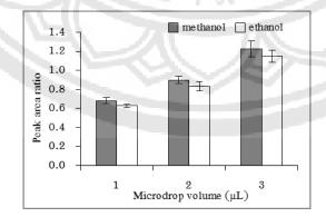
Figure 2 Effect of microdrop volumes of water extraction solvent on peak area ratio of methanol and erthanol. Error bar was 1S.D. (n = 3).
