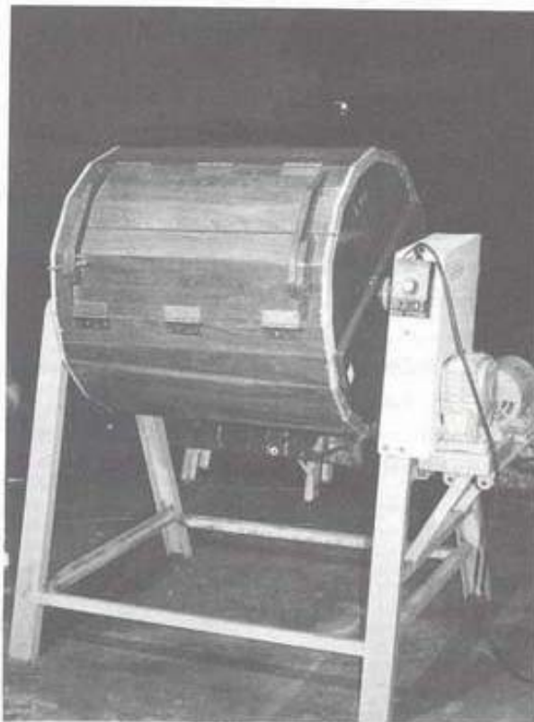
Fig. 2 The compact rotary type of spraying machine with wooden components, containing fishbone wooden structures on the inner wall.
