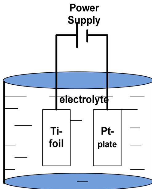
Figure 1. The schematic diagram of a single-face anodization process.
