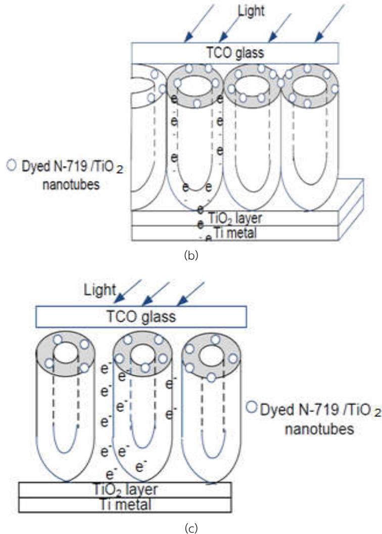
**Figure 6** A schematic diagram of photo-response for dye-sensitized solar cells (b) anodized once and annealed at 450 °C and (c) re-anodized after heat treatment at 450 °C.
