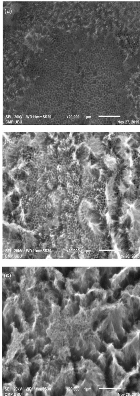
**Figure 3** SEM image (top surface views) of TiO<sub>2</sub> nanotubes with different tops
