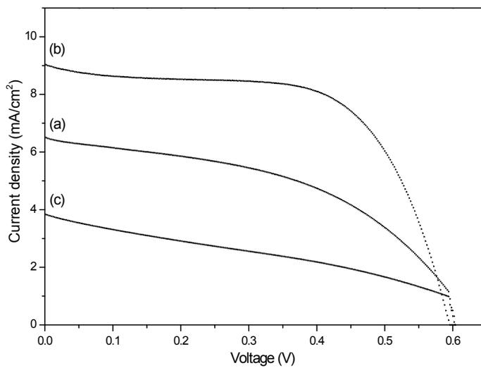
Figure 5 I-V characteristic curves of DSSCs for the samples (a) anodized without heat treatment (b) anodized once and annealed at 450 °C and (c) re-anodized after heat treatment at 450 °C.
