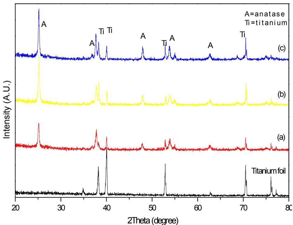
Figure 2. XRD patterns of anodized  $\text{TiO}_2$  nanotubes for samples (a) anodized without heat treatment (b) anodized once and annealed at  $450^\circ\text{C}$  and (c) re-anodized after annealing at  $450^\circ\text{C}$ .
