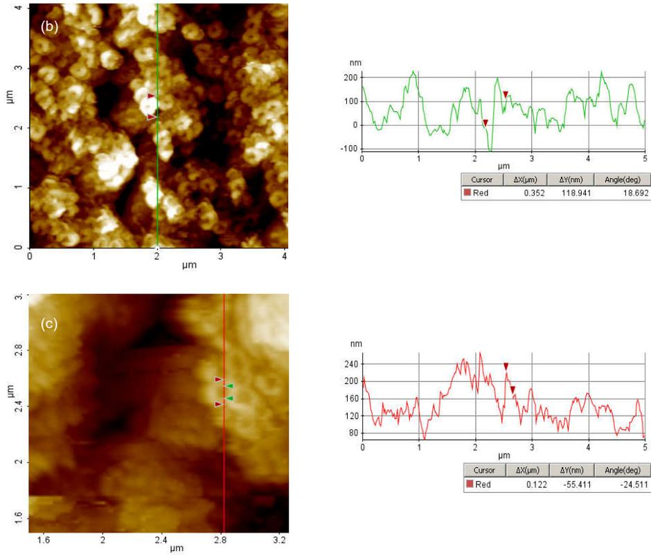
Figure 4 AFM image of anodized TiO<sub>2</sub> nanotubes (b) anodized once and annealed at 450 °C and (c) re-anodized after heat treatment at 450 °C.
