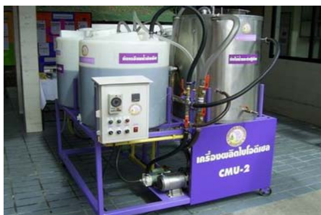
Figure 1. A demonstration of biodiesel unit from used vegetable oil developed by ERDI.
