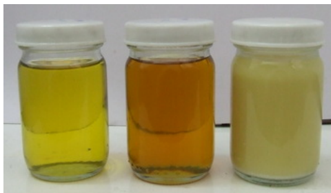
Figure 6. Comparison of emulsified oil with diesel oil and transestered biodiesel (Diesel oil, Transestered biodiesel, Tung oil/diesel/water emulsion, respectively).
