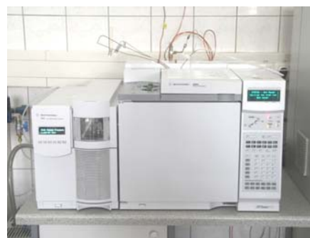
Figure 2. GC-MS system for identification and quantification of trace gas compounds.
