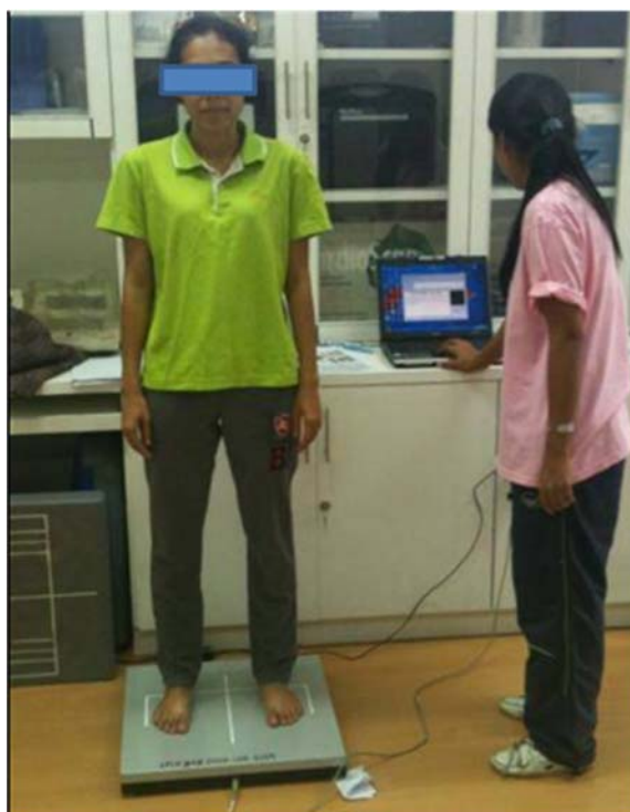
Fig. 1 Balance checker, AM Bertec, Columbus, a static balancing ability on both normal and soft surfaces on force plate. The balance is checked by a software balance check TM screener and trainer 3.3.2 by BERTEC Columbus.
