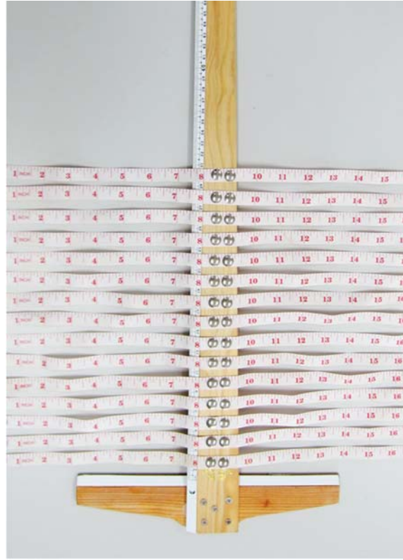
Fig. 1 The customized T-square ruler installed perpendicularly on the longitudinal bar with plastic tape measures at 2-centimeter intervals spanning for 30 centimeters from the shorter bar.
