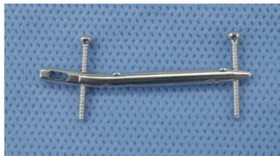
Fig. 1 Prototype of metacarpal locked intramedullary nail with 3 mm in diameter and 45 mm in length. Locking screws are 1.5 mm in diameter.
