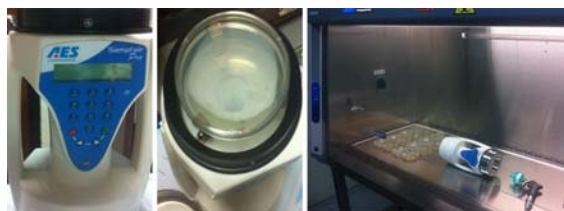
Fig. 3 Microbial air sampler and active air samplings in biological safety cabinet.
