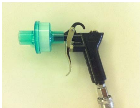
Fig. 2 Reusable sterile hand piece and microbial air filter at the end of the sprinkler.
