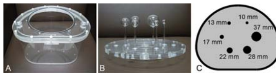
Fig. 1 (A) NEMA PET body phantom, (B) the circular cover with six spheres attached and (C) a cross section of the NEMA PET body phantom with six spheres
