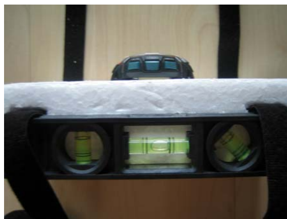
Fig. 2 A fluid base inclinometer with a digital compass angle finder mounted on the stable platform
