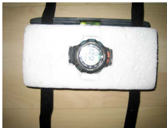
Fig. 3 A top view of the designed instrument, note an inclinometer along the side and a digital compass angle finder on the top of the platform with a Velcro strap
