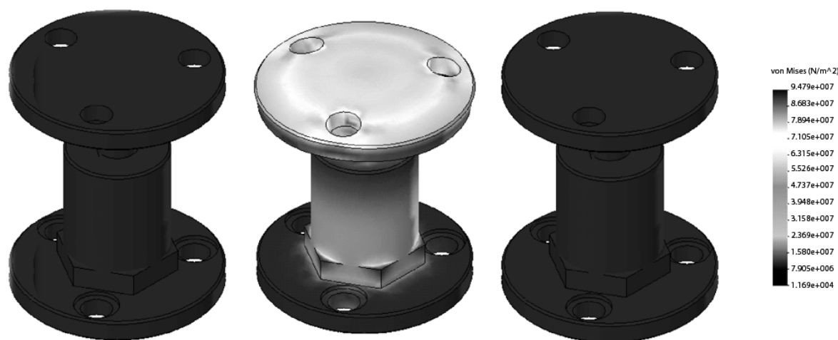
Fig. 8 Dynamic compressive loading on the device (left: initial phase of compressive loading, center: mid phase of maximal compressive loading (1250 N) and right: late phase of unloading of the device)
