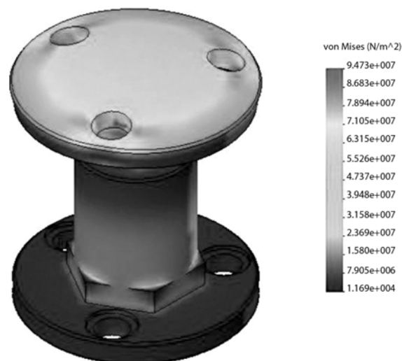
Fig. 7 Stress distribution in the device while compressive load of 1250 N is applied
