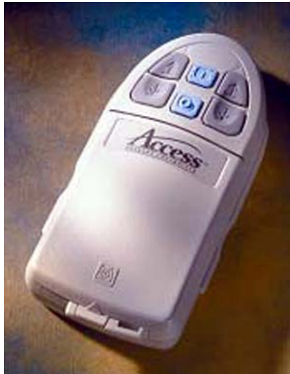
Fig 6. Access Review Therapy Controller. The patient can place this compact controller over the neurostimulator and presses buttons to turn the neurostimulator ON and OFF (With permission from Medtronic)
