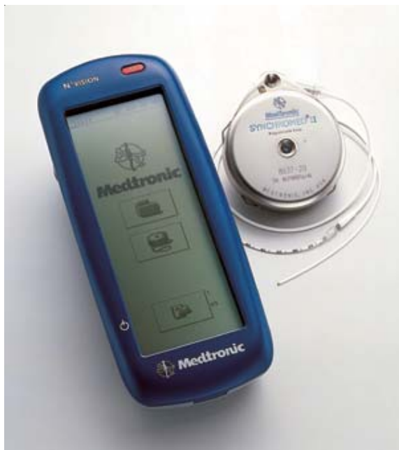
Fig. 5 Physician programmer. Physicians use the programmer to adjust the stimulation parameters noninvasively (With permission from Medtronic)
