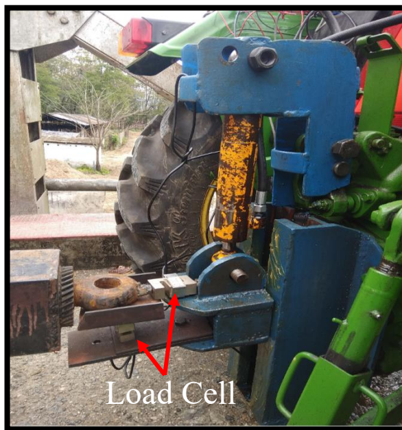
Figure 2. Load cells arrangement to measure draft and vertical force
