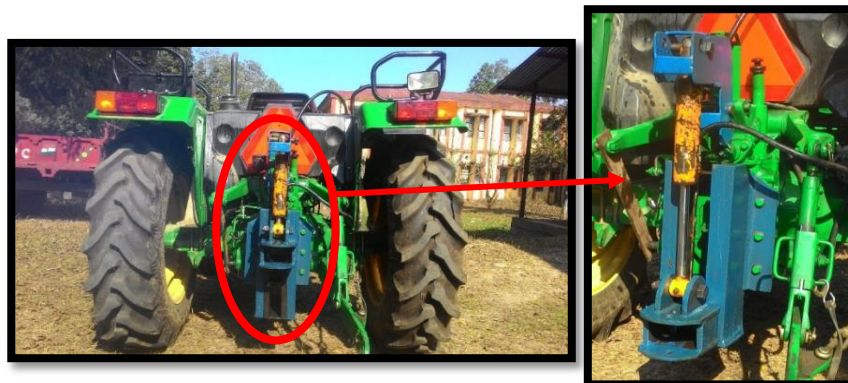
Figure 1. Hydraulically controlled variable single hitch point of test tractor
