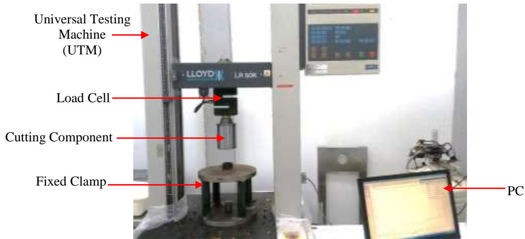
Figure 1. The Universal Testing Machine (UTM) with maximum force of 50 kN and its main components
