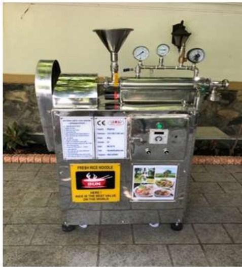
Figure 12. Proposed fresh Bun making machine prototype
