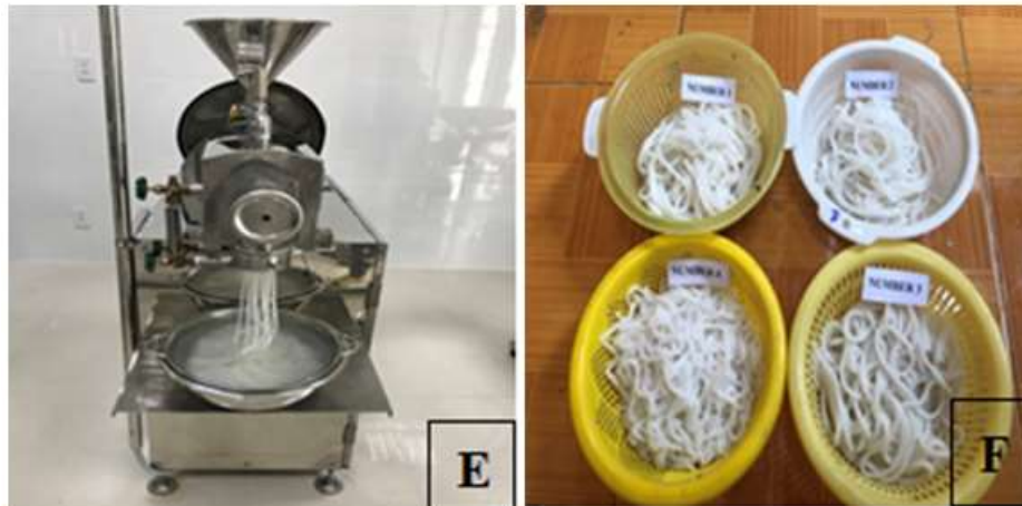
Figure 13 E-Small sized machine in the process of making Bun , F-Produced fresh Bun
