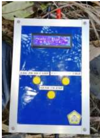
Figure 2. A newly developed impedance meter for measuring soil water content using the dielectric method in the field
