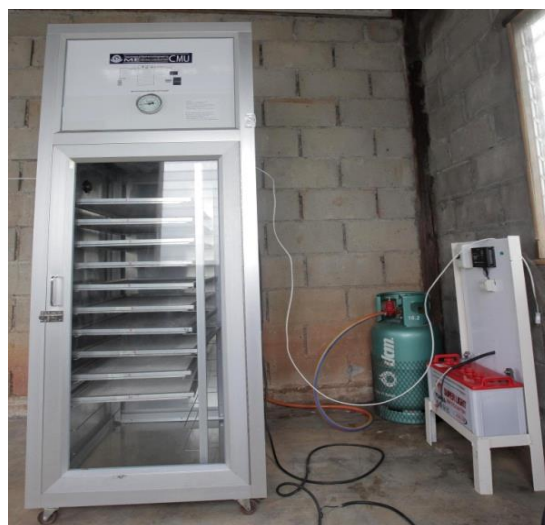
Fig. 1. An LPG cabinet dryer that uses solar energy
