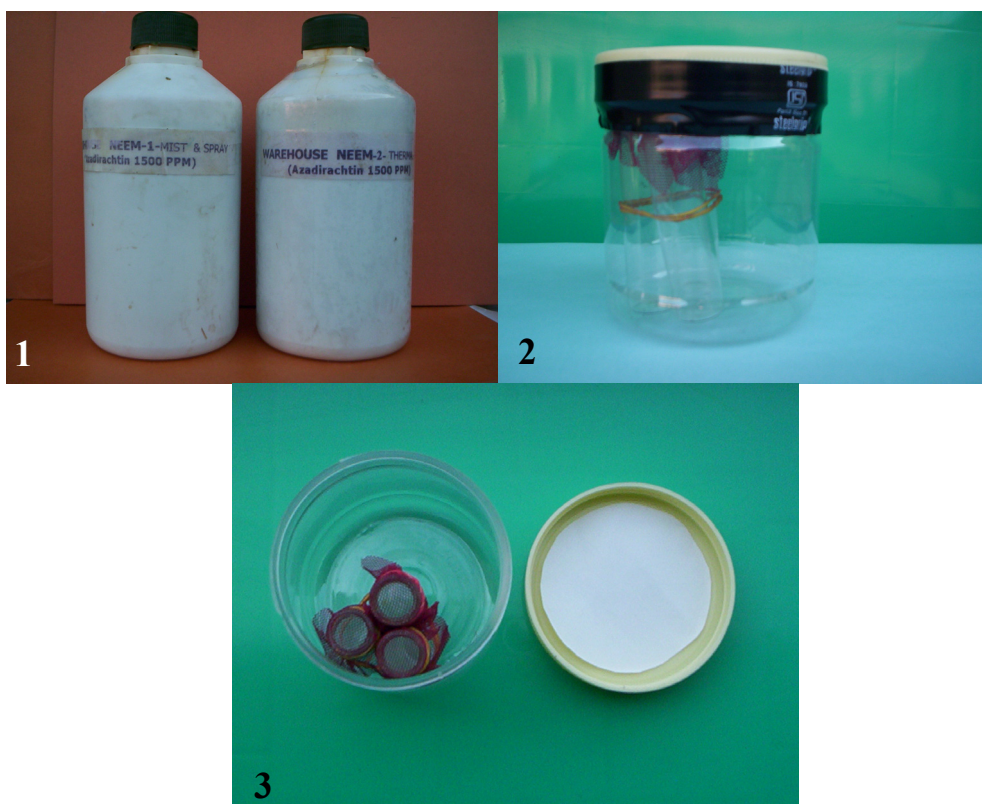
Fig. 1. Neem formulations WHN I and II used in the present study. Fig. 2. Fumigation chamber containing glass vials covered with net and lid with filter paper. Fig. 3. Sealed fumigation chamber to create airtight condition.
